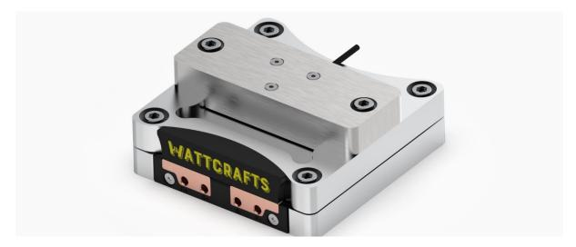
The Force Sensor Module is an advanced attachment designed to enhance the capabilities of our Pouch Cell Holder. This device allows for accurate force measurement and control during battery testing, enabling studies on the effects of pressure on cell performance, safety, and longevity. The module seamlessly integrates with our Pouch Cell Holder, providing either real-time force data or the ability to set precise initial pressures for your experiments.
