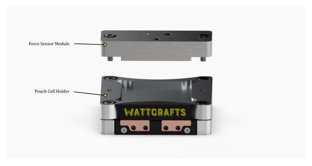
To use Force Sensor Module, mount it into the Top frame of Pouch Cell Holder with 2 socket head screws. It is recommended to do this before tightening the 4 corner screws. This way the initial pressure can be monitored during the assembly. After assembly the module can be used to monitor the pressure evolution in the cell during operation.
