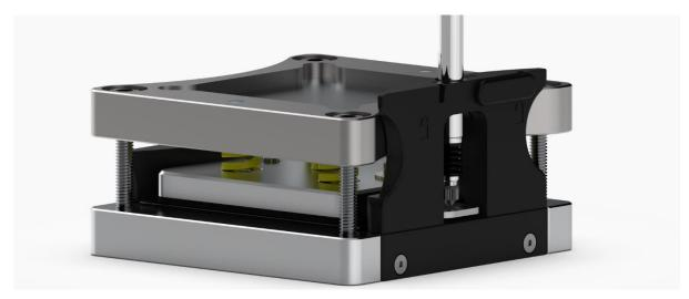
The Thickness Sensor Module is a precision measurement attachment designed to complement our <u>Pouch Cell Holder</u>, offering unprecedented accuracy in tracking battery cell volume changes during electrochemical testing. The module delivers ultra-precise displacement measurements with a resolution of 0.1  $\mu$ m and an accuracy of 1  $\mu$ m across a 5 mm measurement range. This level of precision allows getting insights into single layer prototypes, and up to multilayer commercial cells.
