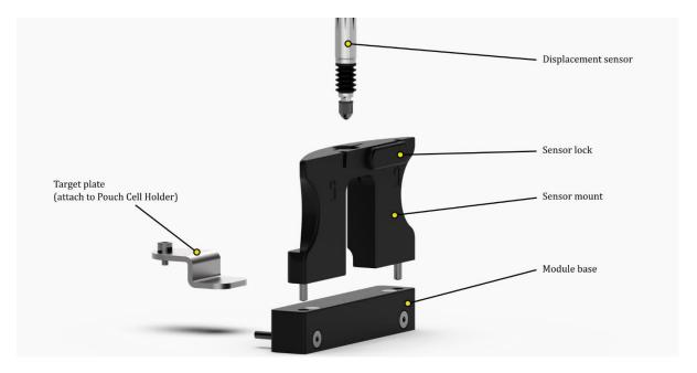
The Thickness Sensor Module is mounted on the back of the Pouch Cell Holder, opposite the electrical contacts. It replaces the back guiding element normally mounted there. The module consists of 4 main elements: target plate, base, sensor mount and displacement sensor. Thickness sensor module should be only used in the 'fixed pressure' mode, i.e. with springs (see Pouch Cell Holder manual).
