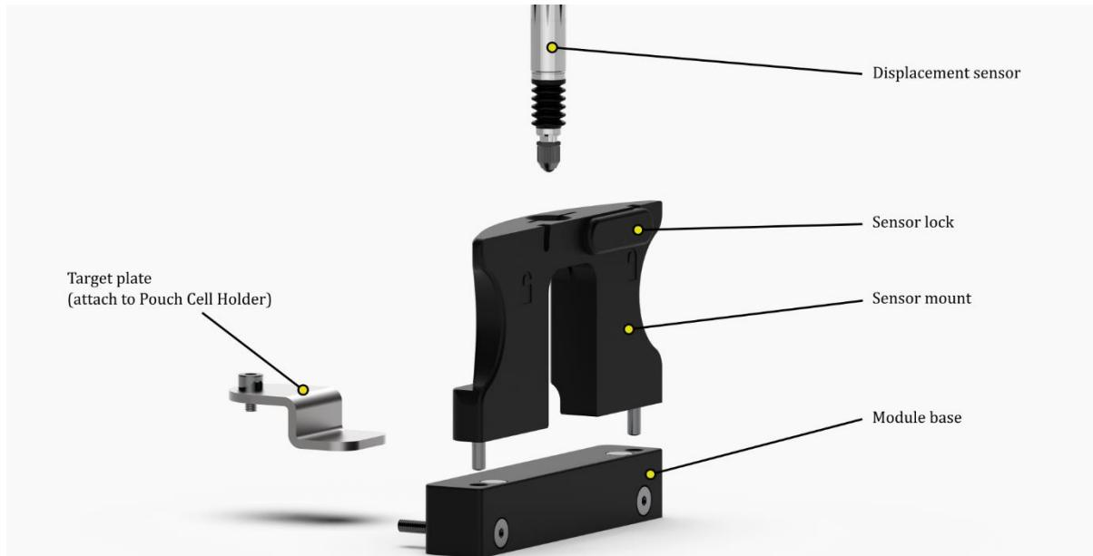
The Thickness Sensor Module is mounted on the back of the Pouch Cell Holder, opposite the electrical contacts. It replaces the back guiding element normally mounted there. The module consists of 4 main elements: target plate, base, sensor mount and displacement sensor. For best results the Thickness Sensor Module should be used in the 'fixed pressure' mode, i.e. with springs (see Pouch Cell Holder manual).
