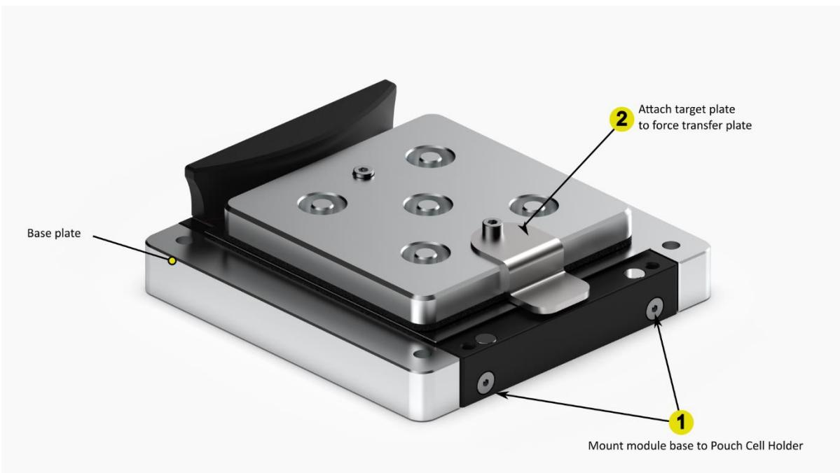
1. Unscrew two screws of the back guiding element on the pouch cell holder base and use them to attach module base in the same place.
