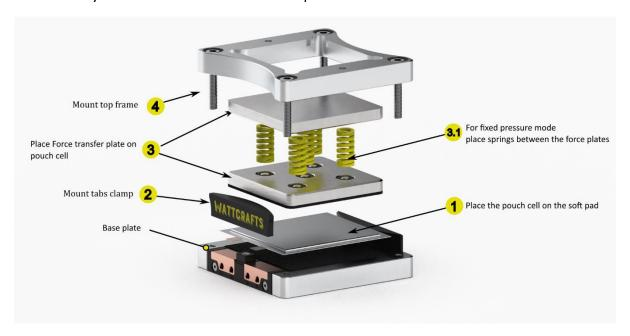
1. Place the pouch cell on the soft pad of the base plate. Align the top cell edge (with tabs) to the plastic cubic block (see below). Make sure that the cell is placed on the correct side to ensure right polarization.
