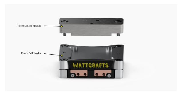
To use Force Sensor Module, mount it into the Top frame of Pouch Cell Holder. It is recommended to do this before tightening the 4 screws (step 4 above). This way the initial pressure can be monitored during the assembly. However, the Force Sensor Module can be attached to the holder at any stage, even during cycling or after finished measurement to check the current pressure applied to the cell.
